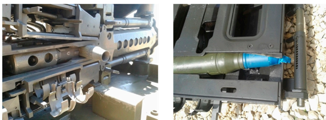
Figure 3. Example of a technical inconvenience for cal. 25 mm machine gun: jammed munitions during the feeding cycle).
